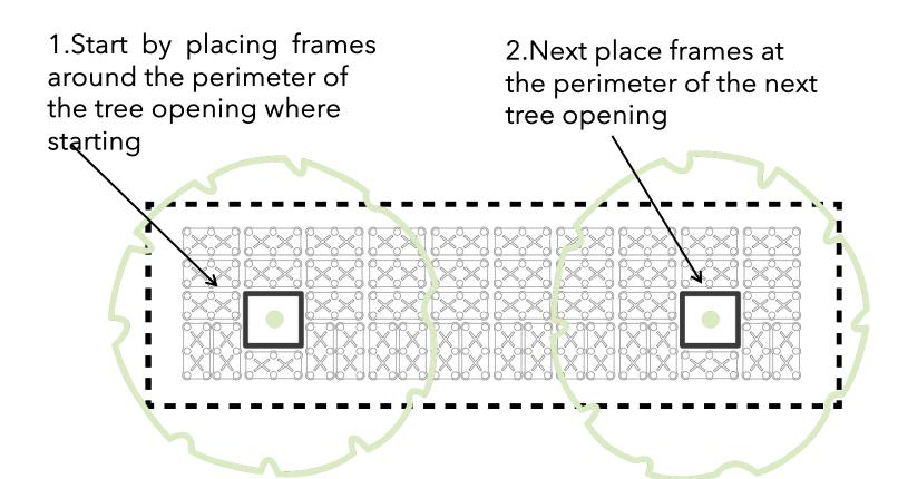
3.Then fill in-between using the quantity of Silva Cells shown in the drawings and space accordingly. The minimum space is 25mm. The maximum space should not exceed 150mm.
