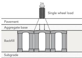
The Silva Cell has been meticulously engineered to handle multiple competing needs, including paving and related vehicle loads, providing maximum space for unimpeded soil volume, and ease of construction – including placement within areas of high services and utility infrastructure. We have years of in-ground projects in multiple applications, providing examples of daily use in high demand environments. For more details please contact us to discuss applications for your project.
