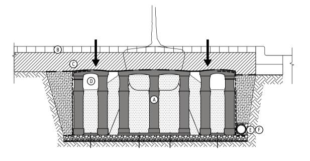
SILVA CELL SYSTEM + PERMEABLE PAVEMENT
