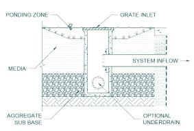
NOTE: SWALE AND BIORETENTION ROAD VERGE CONFIGURATIONS POSSIBLE.
