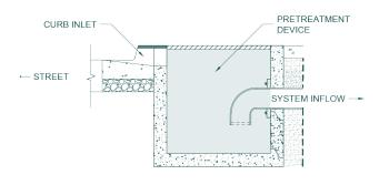
NOTE: PRETREATMENT DEVICE INSTALLED PER MANUFACTURER RECOMMENDATIONS. OPTIONS INCLUDE HYDRODYNAMIC SEPARATORS, FILTRATION DEVICES, AND FLOW REGULATORS.
