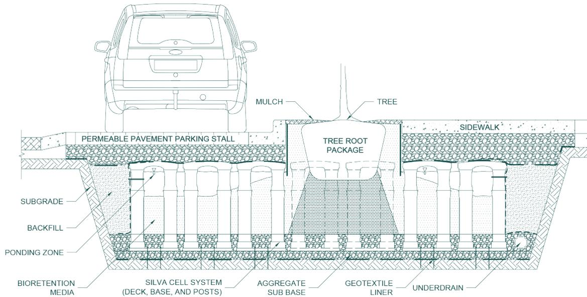
NOTE: MEETS AASHTO HS-20 (USA) CSA-S6, 87.5 AND OBC 54KN (CANADA), AND BS EN 1991-1-1:2002 BS EN 1991-1-2:2003 (UK) LOADING STANDARDS WHEN USED WITH STANDARD PAVING PROFILES. INCREASED LOADING CAPACITY CAN BE ACHIEVED BY ADJUSTING THE STANDARD PROFILES.
