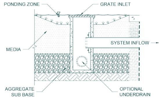
NOTE: SWALE AND BIORETENTION ROAD VERGE CONFIGURATIONS POSSIBLE.
