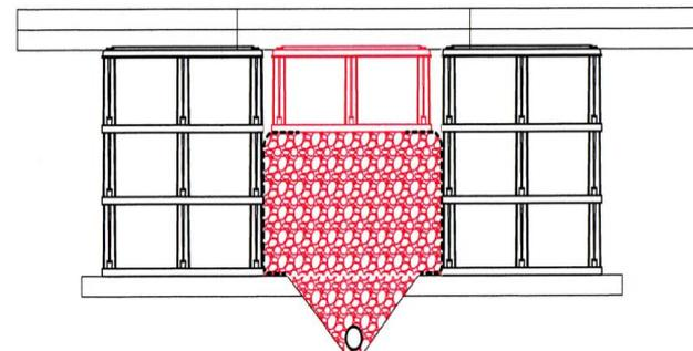
**Option 3** – fill/compact the excavation to the bottom of the Silva Cells, install geogrid around the perimeter of the remaining opening and fill with compacted soil, clear stone or flowable fill/U-fill (in the case of flowable fill, try to establish some link between adjacent soil volumes)
