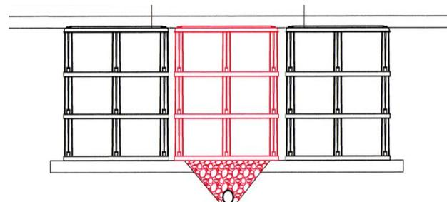
**Option 2** – fill/compact the excavation up to the bottom of the uppermost layer of Silva Cells and re install a single layer of frames and decks
