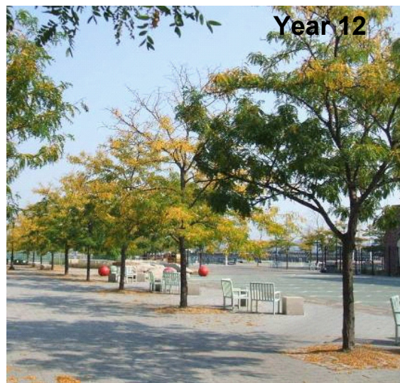
Trees in CU Soil Appr. 175 cf net soil/tree (350 cf of CU Soil)
