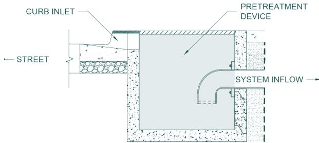
NOTE: PRETREATMENT DEVICE INSTALLED PER MANUFACTURER RECOMMENDATIONS. OPTIONS INCLUDE HYDRODYNAMIC SEPARATORS, FILTRATION DEVICES, AND FLOW REGULATORS.
