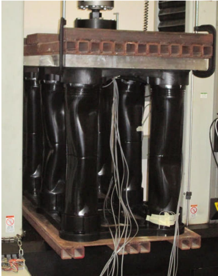
Figure 3: Typical Silva Cell 2X Failure
