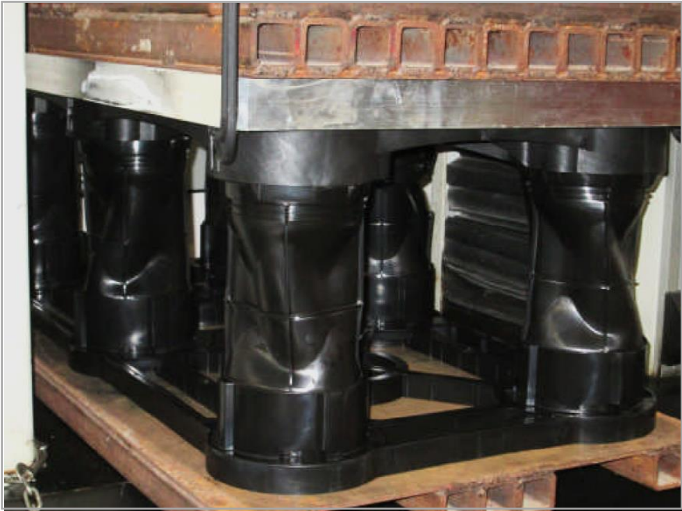
Figure 1: Typical Silva Cell 1X Failure
