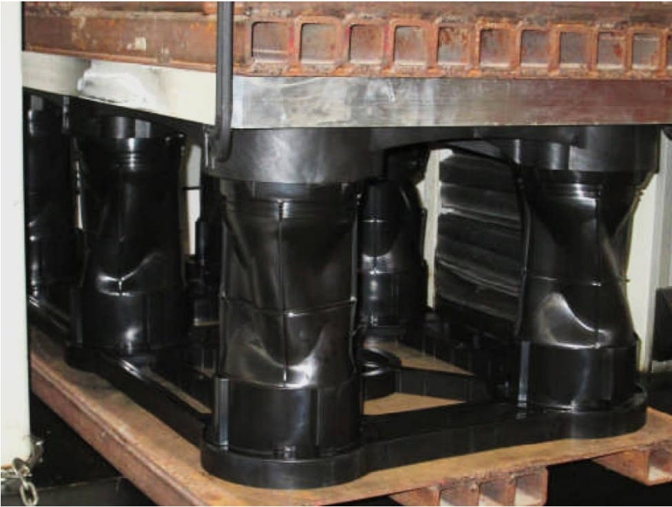
Figure 1: Typical Silva Cell 1X Failure
