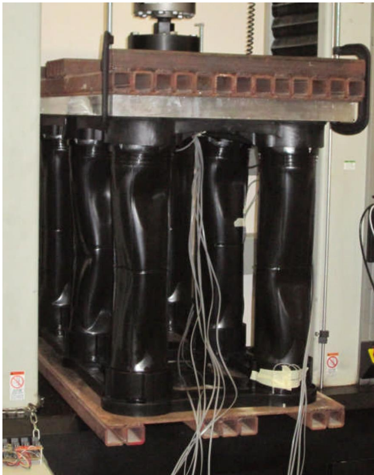
Figure 3: Typical Silva Cell 2X Failure
